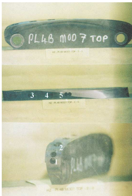
Fig. 3. Sampling points and measured tritium activities on JET graphite limiter tile PL4BMOD 7B TOP. Shown from top to bottom are the lateral, plasma-exposed and front sides, respectively. The concentrations in the first mm depth are 3.8 (1), 592.05 (2), 290.51 (3), 42.77 (4) and 12.61 MBq/cm 2 (5).
